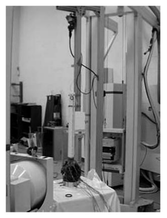
*Fig. 3.* Specimen attached to impact fixture and positioned in front of high-speed biplanar X-ray machine.
